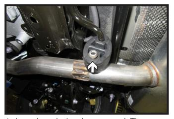
3. **Optional/Some Models**: Support center exhaust pipe using a jack or bungee cord. Then remove rubber isolator from exhaust rod.
