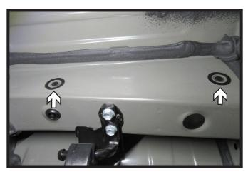
Remove the stickers covering the holes in the side for the frame. Do this on both sides of the vehicle.
