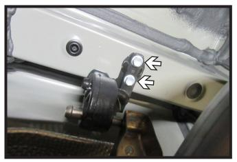
2. **Optional/Some Models**: To allow for clearance and easier hitch installation, lowering the exhaust may be needed. Support exhaust, then using a 12MM socket, remove the two (2) bolts from the exhaust hanger. Do this on both sides of the vehicle.
